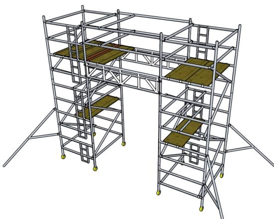
**11** Repeat Step 9 for either three, four or five decks depending on the length of beam unit used.
