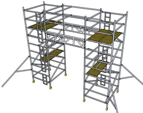
**9** Working from one tower slide an appropriate length fixed platform under the tower side handrail to rest on the beam units, approx 150mm gap between the tower deck and the deck on the beams
