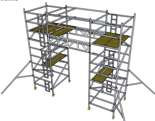
**10** Fit a beam unit infill deck to bridge the gap between the tower deck and the beam unit deck, some slight adjustment may be necessary to ensure a snug fit.
