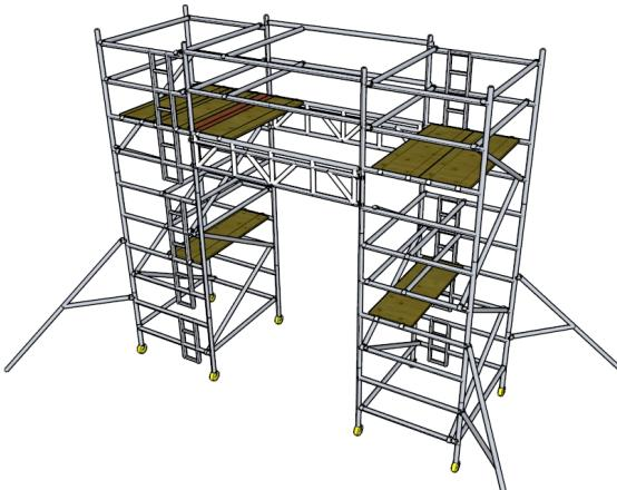
**12** When all the decks are positioned on the beams fit the second beam unit infill deck to close the gap between the beam decks and the tower deck, some slight adjustment may be necessary to ensure a snug fit.
