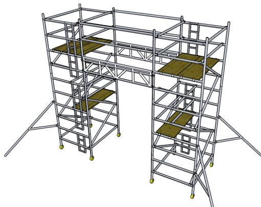
**8** Working from 1 tower fit an extra pair of horizontal braces to suit the size of tower being used, position on the upper and lower beam unit handrail braces to the offside of the deck resting on the beams. This will provide double handrail protection on the beam unit platform as decks are positioned
